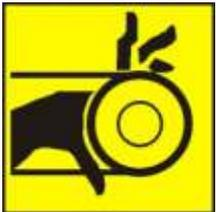
This warning symbol alerts you to the presence of possible dangerous drive mechanisms within the machine. Guards should always be in place when the machine is in operation.
